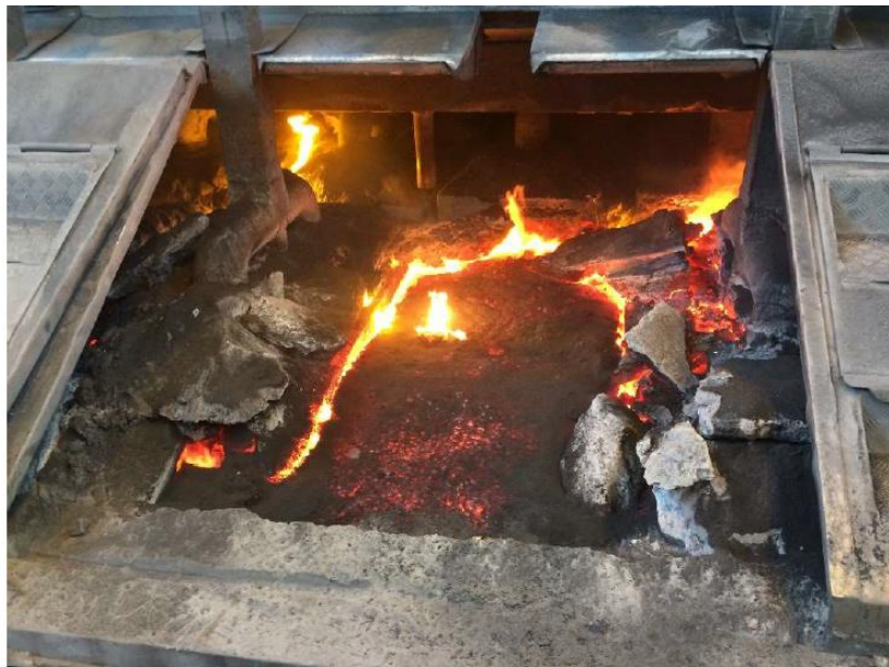
Figure 6. Cell with extreme dust and excess carbon consumption: Cell 124, 31 May 2018, bath temperature 1072 °C; had to be shut down on 21 June 21 2018 at 1120 °C.
